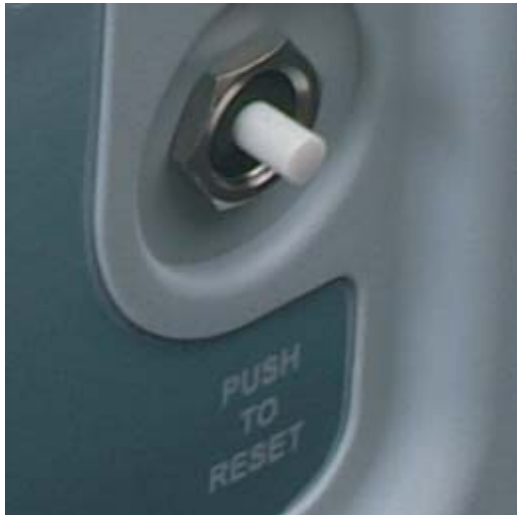
Circuit Breaker Reset
